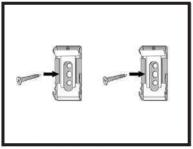
1.Install the two brackets on the wall with screws provided.
