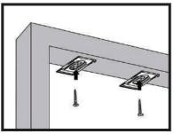
1.Install the brackets on the ceiling with screws provided.
