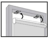
2.Hook the rail onto the bottom of the bracket and rotate it until the back of the rail securely snaps into place.
